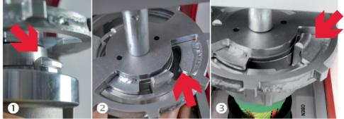
The notch of the outer ring must be placed in the form.
